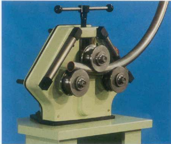
Optional roll sets may be used to roll tubes up to 2 3 / 8 inch diameter.
