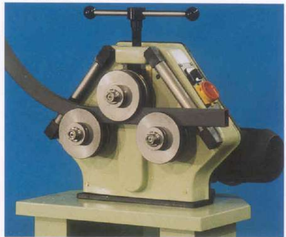
Square or rectangular tubes, larger than 1 1/4", require optional roll discs for added support to tube walls.
